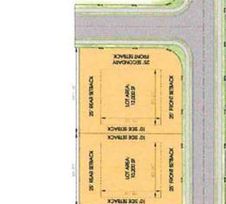
(R-1) 100-FT WIDE TYPICAL LOT DIAGRAM N.T.S. 15,000 SF MINIMUM LOTS SIZE 30% MAXIMUM LOT COVERAGE 35-FT MAXIMUM BUILDING HEIGHT (3-STORIES MAX.)
