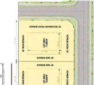
(R-3) 75-FT WIDE TYPICAL LOT DIAGRAM N.T.S. 7,500 SF MINIMUM LOTS SIZE 35% MAXIMUM LOT COVERAGE 35-FT MAX. BUILDING HEIGHT (3-STORIES MAX.)
